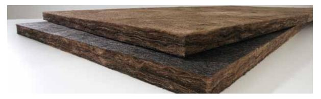
**AKOUSTI-LINER R<sup>TM</sup>** insulation is a heavy-density fiberglass board insulation product made from inorganic glass fibers bonded by a thermosetting binder. Its base board is brown with a black mat facing on the airstream surface.
