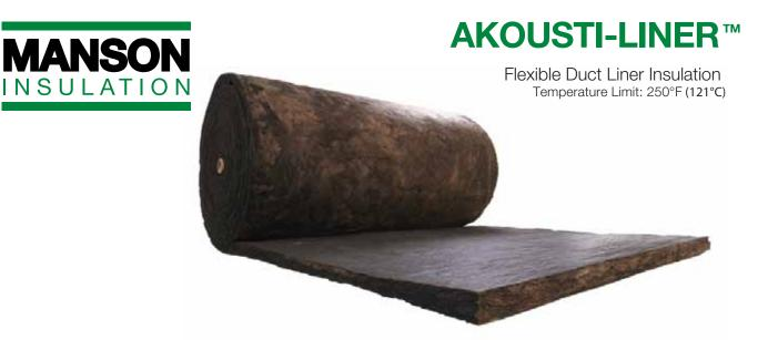
**AKOUSTI-LINER<sup>™</sup>** insulation is a flexible duct liner providing both thermal and acoustical insulation. It is manufactured from inorganic glass fibres bonded with a thermosetting binder. The airstream surface is faced with a black mat bonded to the black fiberglass substrate. AKOUSTI-LINER<sup>™</sup> insulation is offered with or without edge coating to seal fibres.
